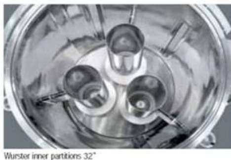
Fig. No.2.3A: Pilot Scale Studies (40 kg each) using 18'' Wurster HS insert
